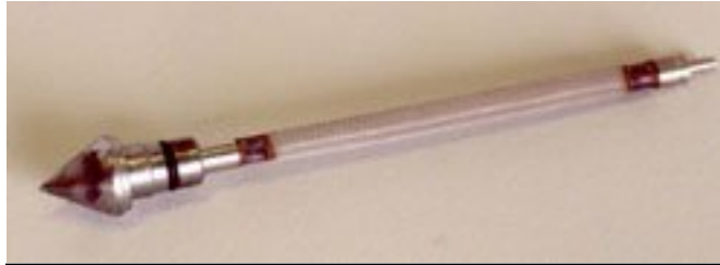
Photograph 7 – Stainless-steel mesh soil vapor point
