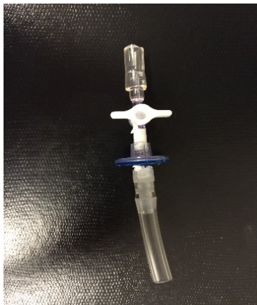
Photograph 9 – Inline moisture filter and stopcock assembly (See Photograph 13, Item [C])
