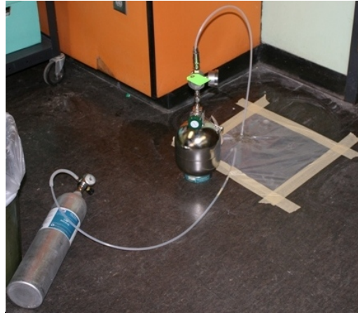
Photograph 21 - Plastic wrap leak detection method during sampling
