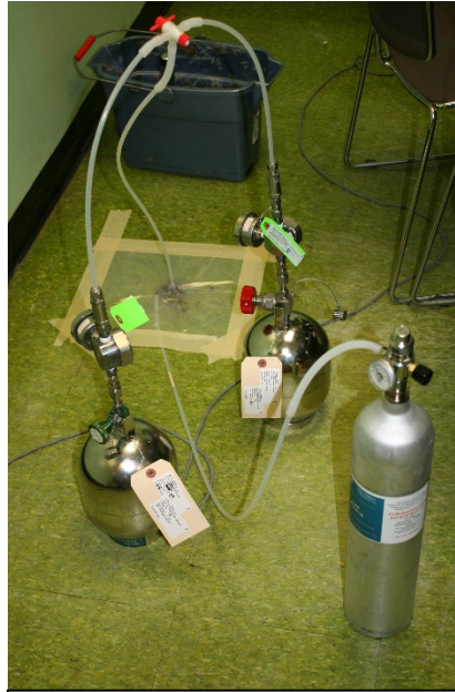
Photograph 15 - Field duplicate sample collection setup
