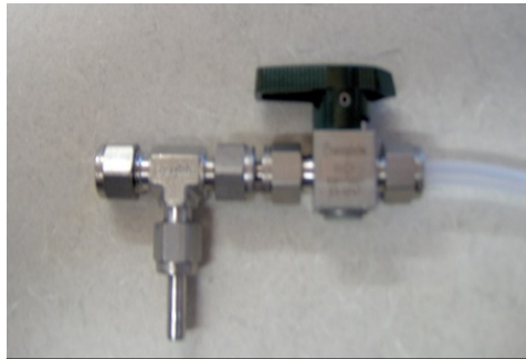
Photograph 17 - T-connection for quantitative tracer gas testing
