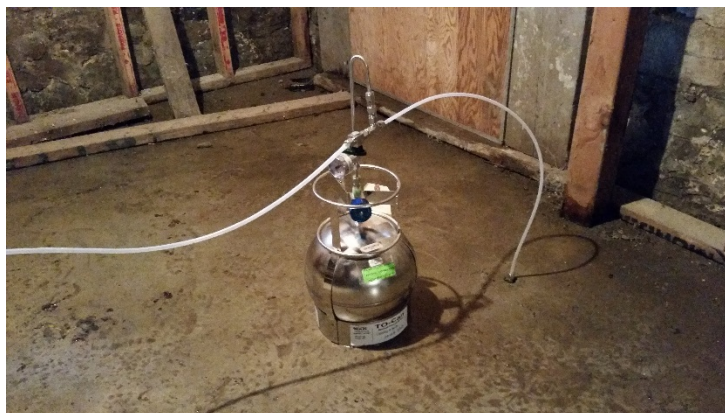
Photograph 6 – Sample collection at temporary sub-slab vapor point
