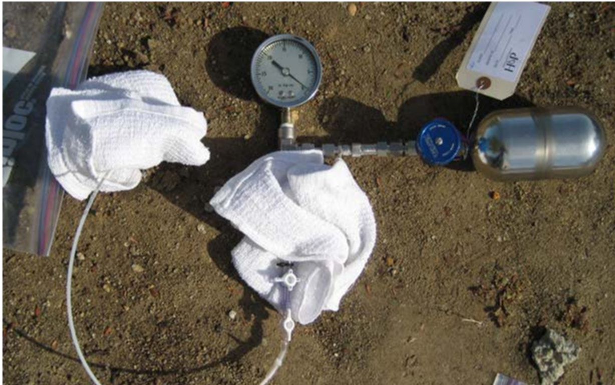
Photograph 19 - Soil gas sampling set up with semi-quantitative leak testing applied via rags draped over vapor point and sampling apparatus. Note: Although rags are placed around fittings here, a single rag placed immediately adjacent to the sampling apparatus is sufficient when using the Rag Method to apply a semi-quantitative tracer.
