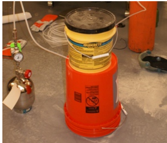
Photograph 22 - Inverted container leak detection method with helium tank in background (right). Leak detection for vapor point only, canister outside of container.
